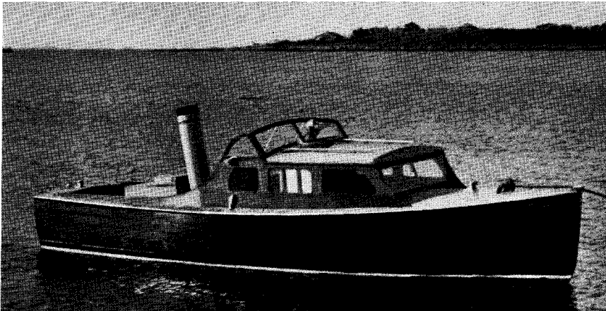
Figure 1. Hero II at mooring. The hatch aft of the stack houses the boiler. Engine is forward, under floor.
