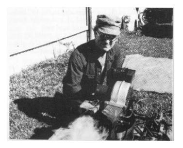
mounted on bricks with a wood fire. This worked well on 25 psi with a small fire.
