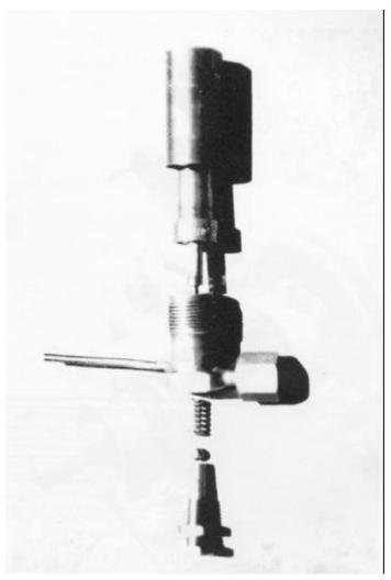
A Bosch 15S2 pintle nozzle is used in this modified injector. This is used in direct firing burners and in conjunction with the pot burner.
