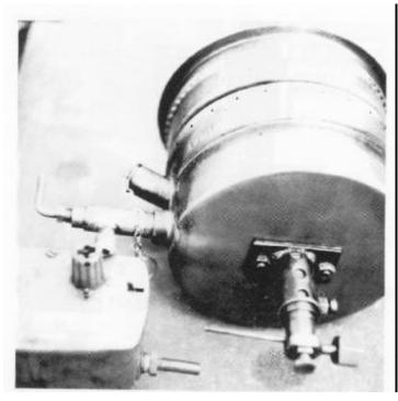
The pot burner is fed by the boxy oil control valve which controls pilot flame size. The central injector has been added and is fed combustion air above the pot burner.
